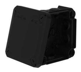
Junction box for the connection of cables and lines indoors and in protected outdoor areas. Square design with plug-in seals to the sides and knock-out entries in the bottom. Suitable for wall and ceiling mounting and on mounting panels. With the option to fasten inside and to mount via the corner domes. Cover with quick lock, sealable. Made from halogen-free and UV-resistant materials.
