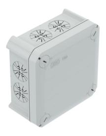
Junction box with strain relief entries for the connection of cables indoors and in protected outdoor areas. Square design with knock-out entries to the sides and knock-out entries in the bottom. Suitable for wall and ceiling mounting and on mounting panels. With the option of fastening inside and to mount via the corner domes. Cover with quick lock, sealable. Made from halogen-free and UV-resistant materials.
